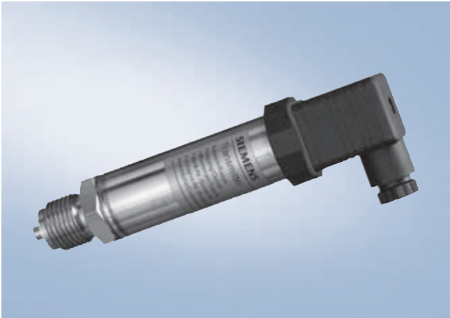
SITRANS P pressure transmitters, Z series for pressure and absolute pressure (7MF1563-...) SITRANS P pressure transmitters, Z series (7MF1563-...), measure the relative and absolute pressure as well as the level of liquids and gases.
